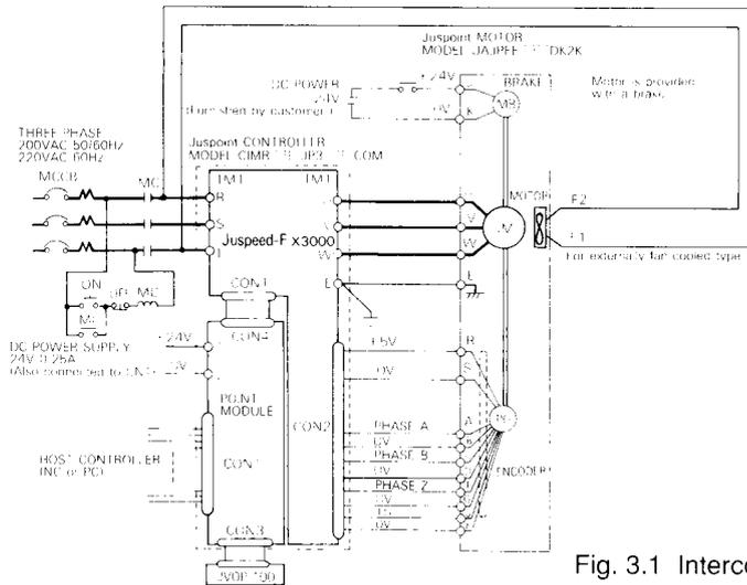
Fig. 3.1 Interconnection Diagram
