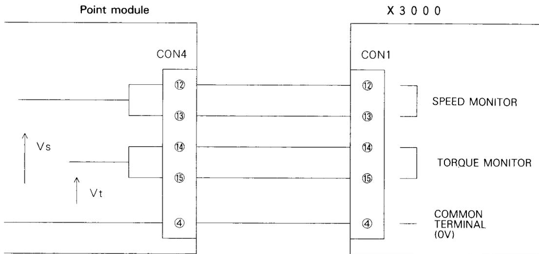
Short terminals 12 - 13 and 14 - 15 and measure the voltage between the common terminal 4 (0V).
