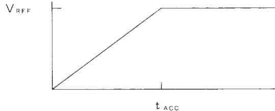
$$t_{ACC} = \text{Acceleration time parameter setting} \times V_{REF} \div 1800 \text{ (msec)}$$
