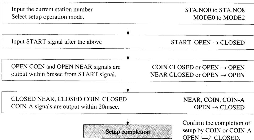
Station number (POS.NO0 to POS.NO8) is output at completion.
