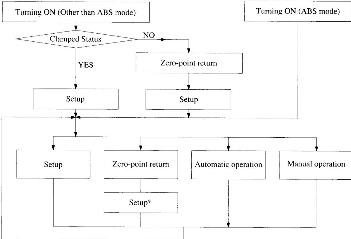
When (C0-15=0), the setup operation is necessary after zero-point return.
