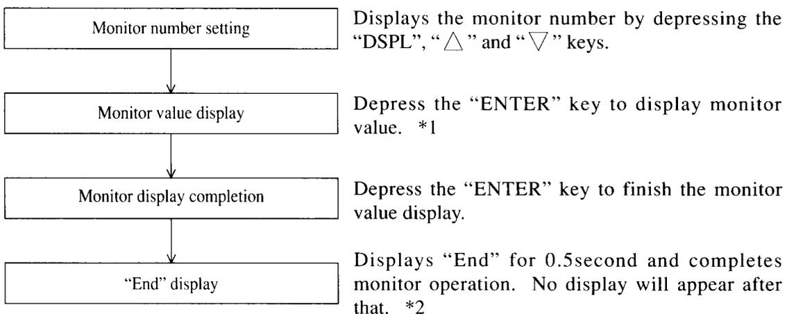
\*1 : Monitoring data during operation shows the changes made every moment (real time).
