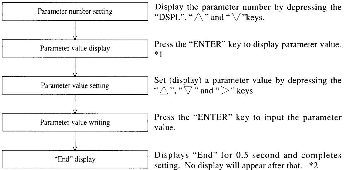
\*1 : Operation will not be possible unless “ENTER” is depressed to finish parameter setting. No operation commands are accepted.
