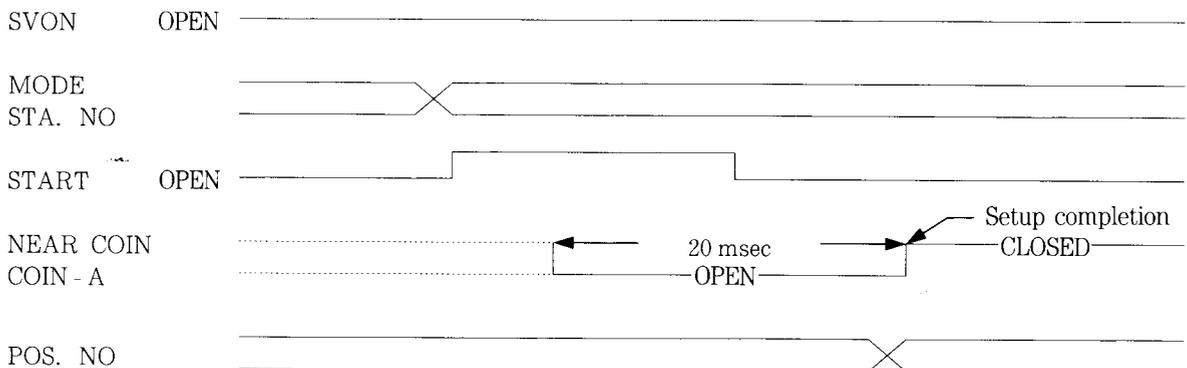
Fig. 4.3 Time Chart of Setup Operation
