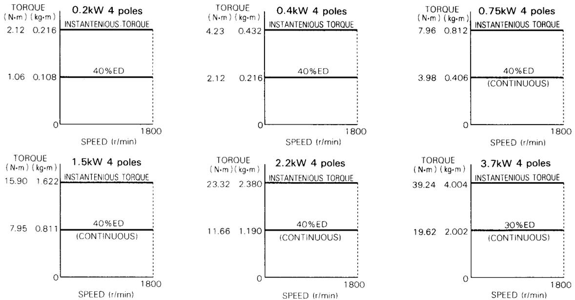
Note : (CONTINUOUS) is externally fan-cooled type.
