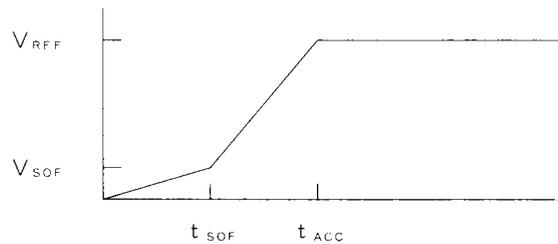
$$t_{ACC} = t_{SOF} + \text{Acceleration time parameter setting} \times (V_{REF} - V_{SOF}) \div 1800 \text{ (msec)}$$
