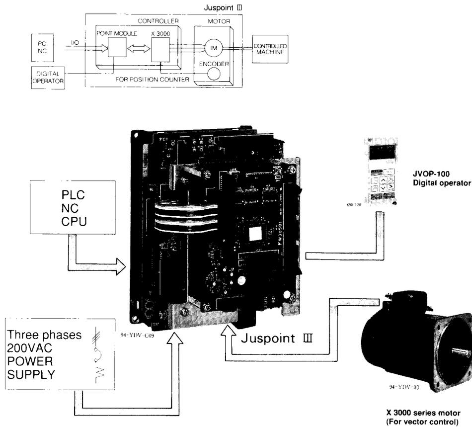
Fig. 1.1 Juspont III System Configuration
